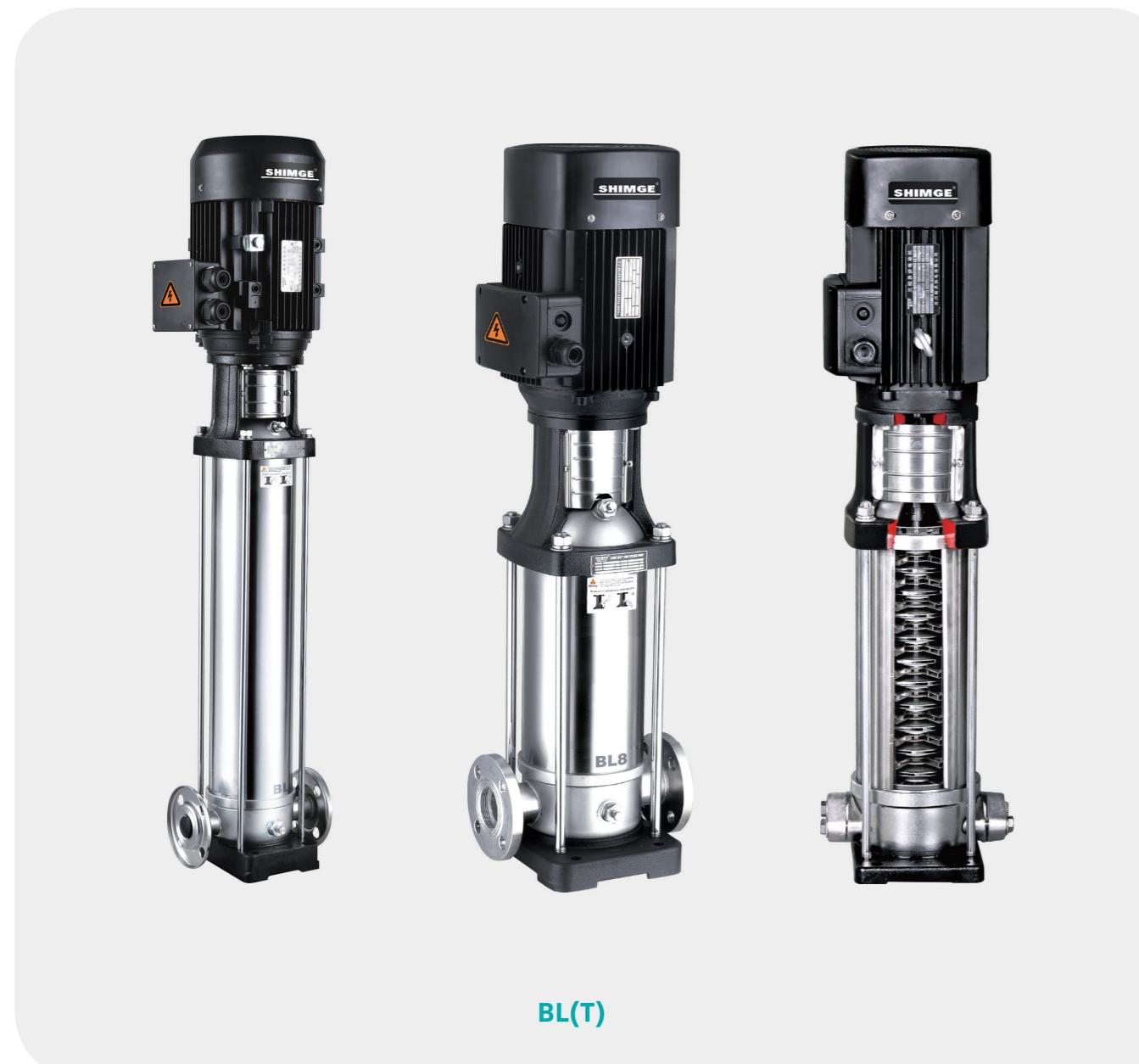
**H**igh-efficiency standard motor, Japan NSK bearings and cold-rolled 50ww800 silicon steel sheet made the pump high efficiency, low noise and maintenance-free. Totally enclosed shaft seal, IP55 protection grade, F class insulation grade, the special "double-lock" drive end bearing made the pump withstand higher inlet pressure.
